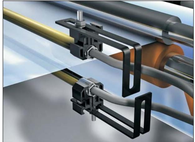
The material web brings along additional electrostatic charge from the machine. With the ionizing bars EI VS in front of the roll the level of static charge can be lowered to a minimum. Fixation possibilities with different types of brackets and bar holders (photos 4 and 5) enable the installation for any machine construction.
