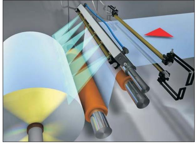
Compressed air containing ions (light blue) flows from the KL VS ionization air lock both onto the small diameter roll (photo 2) and larger diameter roll (photo 3).
